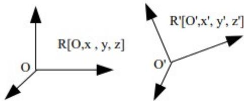
$$\left[ \frac{d\vec{OM}}{dt} \right]_R = \left[ \frac{d\vec{OO}'}{dt} \right]_R + \left[ \frac{d\vec{O'M}}{dt} \right]_{R'} + \vec{\Omega} \wedge \vec{O'M}$$
